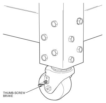
Fig. 11 — Factory-Installed Unit Wheels (4)
